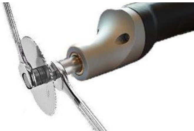
Fig. 1: Releasing the retaining screw
