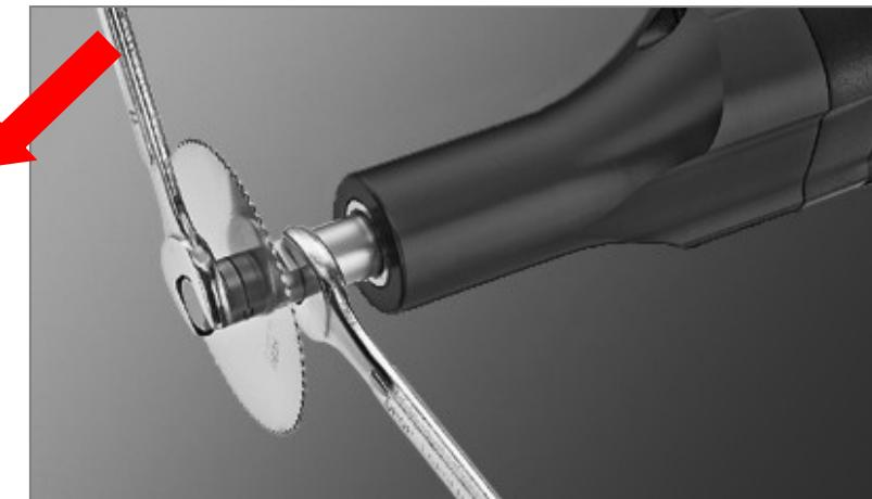
fig. 3 Releasing the retaining screw
