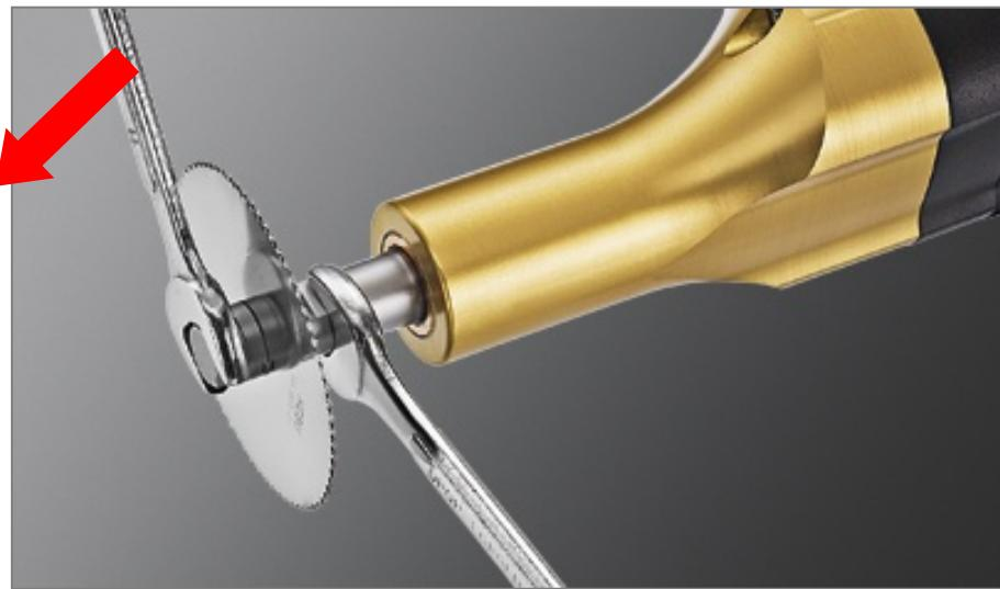
fig. 3 Releasing the retaining screw
