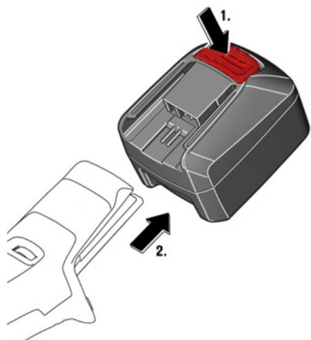
**fig. 1 Removing the accumulator**
