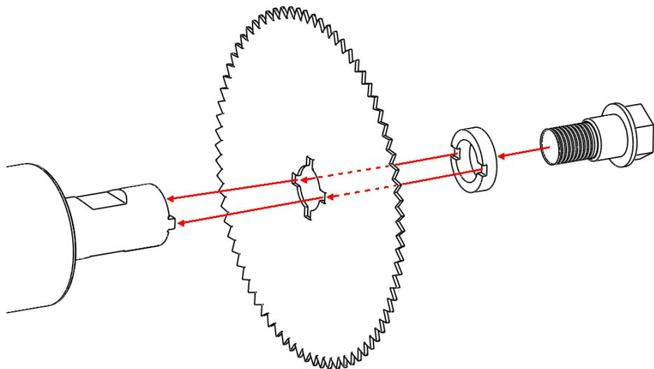
fig. 4 Inserting the saw blade
