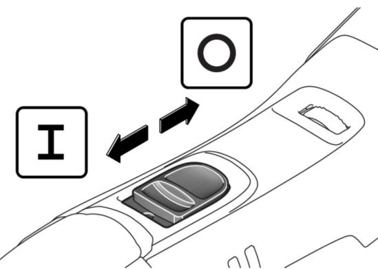
fig. 5 Switching on and off
