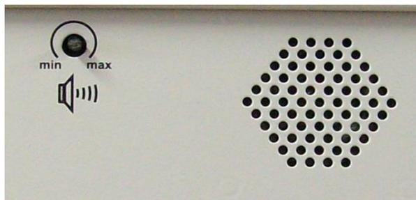
The volume of the activation and message signals can be adjusted using the controller on the rear of the device. The speakers are also on the back. The sounds cannot be turned off.
