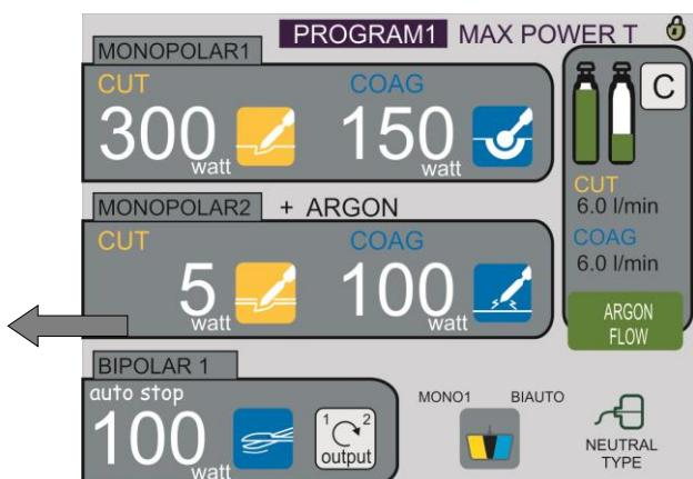
To set the argon function you have to press the "Argon Flow" button on the touch-screen. If it is activate, "+Argon" will appear.
