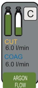
The gas flow can be set at an interval of 0.1 L/min to 6.0 L/min in steps of 0.1 L/min.
