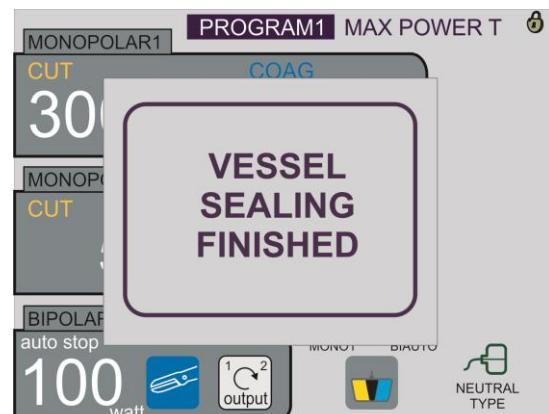
Display: „Vessel sealing finished „– Bi seal mode
