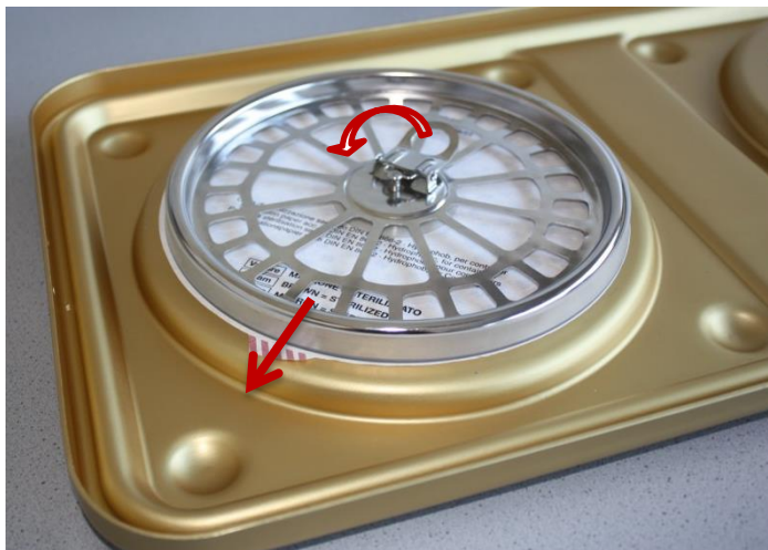
Fig. 2: Filter holder with a paper filter
